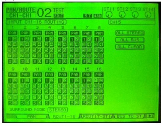
6) In the PAN/ROUTE menu, go to the "ROUTE17-STI" tab. Assign CH32 to the Stereo Buss ONLY and CH32 to BUSS1 ONLY
